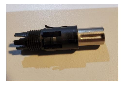
If yo do not seat the pin assembly correctly in the plastic housing, these pieces will not fit correctly in the outer housing.
