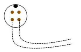
Here is the pinout diagranm for the connector. The two leads **opposite** the alignment groove are the correct leads to used.
