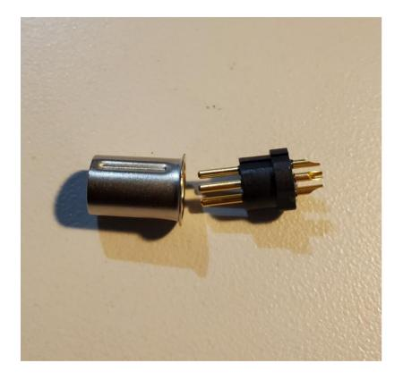
The pin assembly slides into the metal housing. Note that the housing is grooved such that the pin assembly can only fit in in one orientation. Also not that one end of the metal housing is beveled – so note the orientation relative to the pin assembly.
