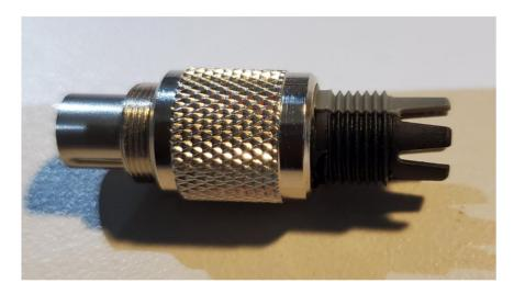
Slide the pin assmbly + inner housing + plastic housing all the way into the outer housing.
