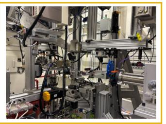
Back spherical analyzer and von Hamos high energy resolution spectrometers
