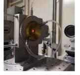
RT-1500°C for electrode material synthesis
